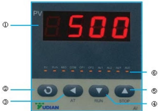
**Basic display status :** When it is powered on, the display window of the instrument shows the process value (PV).
